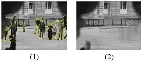
Figure 5: Result on a complex sequence, using downsampling parameters ( n = 10 and p = 4 ). (1) Detection result (contour superimposed on the original image) (2) \Sigma - \Delta mean (used by courtesy of L. Lacassagne UPS/IEF)
